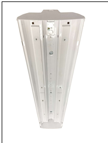
STEP 4 REMOVE BALLAST SOCKET BARS AND ANY WIRING FROM THE LUMINAIRE FOR UP LIGHT LUMINAIRE INSTALL UP LIGHT COVERS (4) 2 FOR EACH SIDE WITH (2) TEK SCREWS PER COVER
